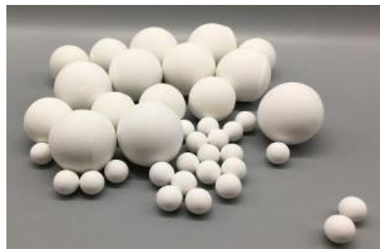
Figure 3.1.2b: High alumina balls
