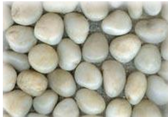
Figure 3.1.2a: Natural pebbles (existing grinding media)
